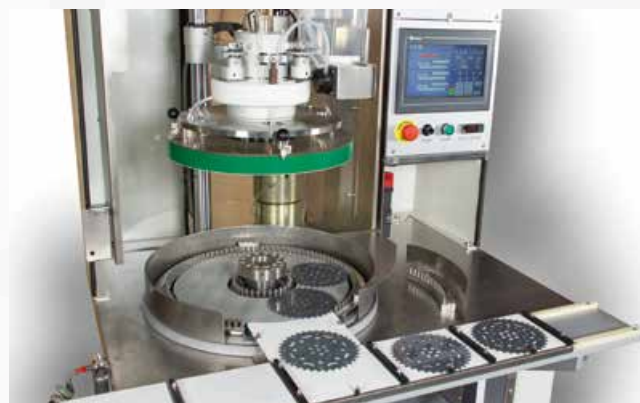
09 2380DE2 0 Satellite unloading system with preparation ramp
