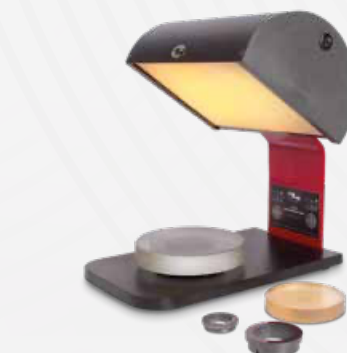
Monochromatic lamp and optical gauges
